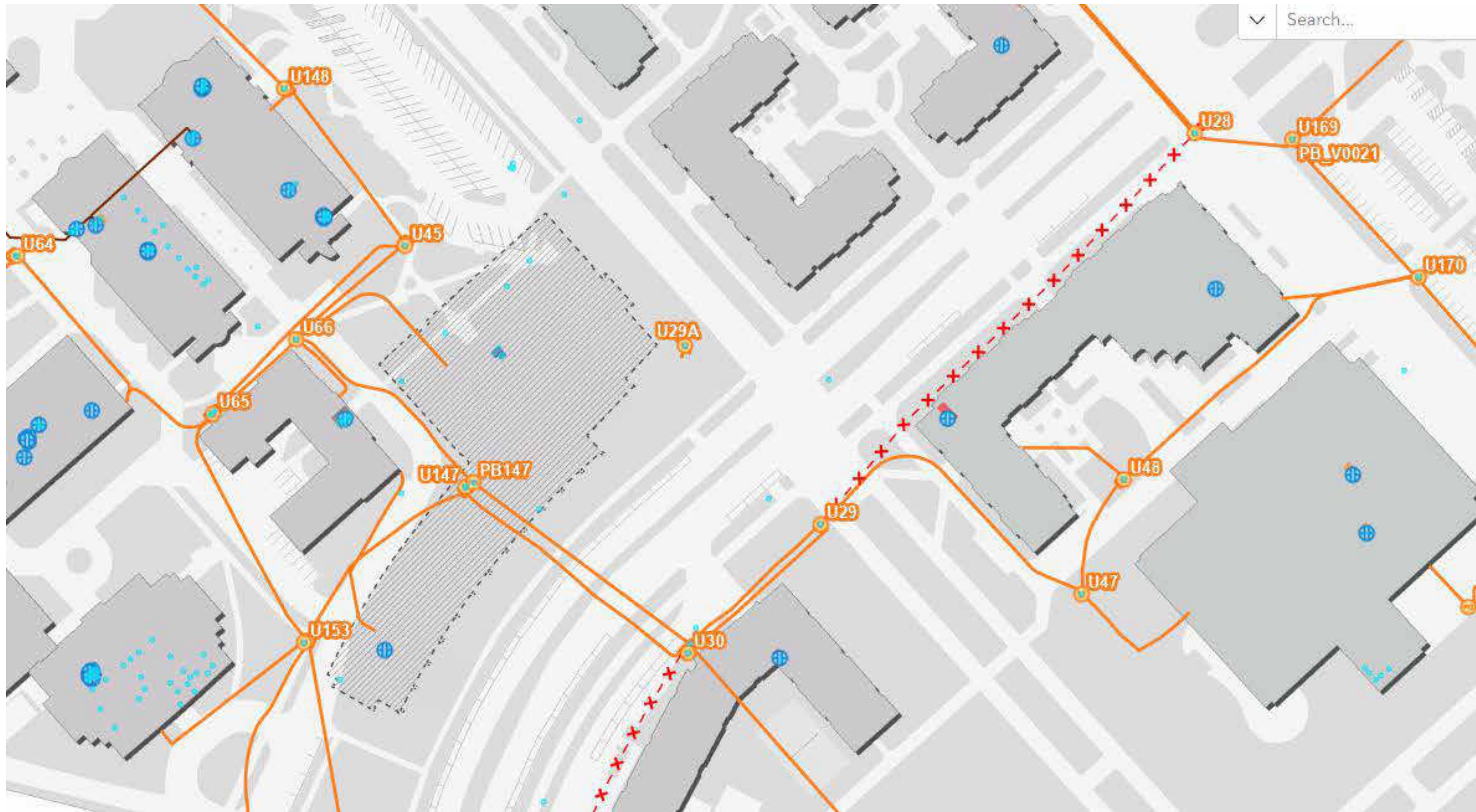
1 EXISTING COMMUNICATION DUCT ROUTING SCALE: NONE
