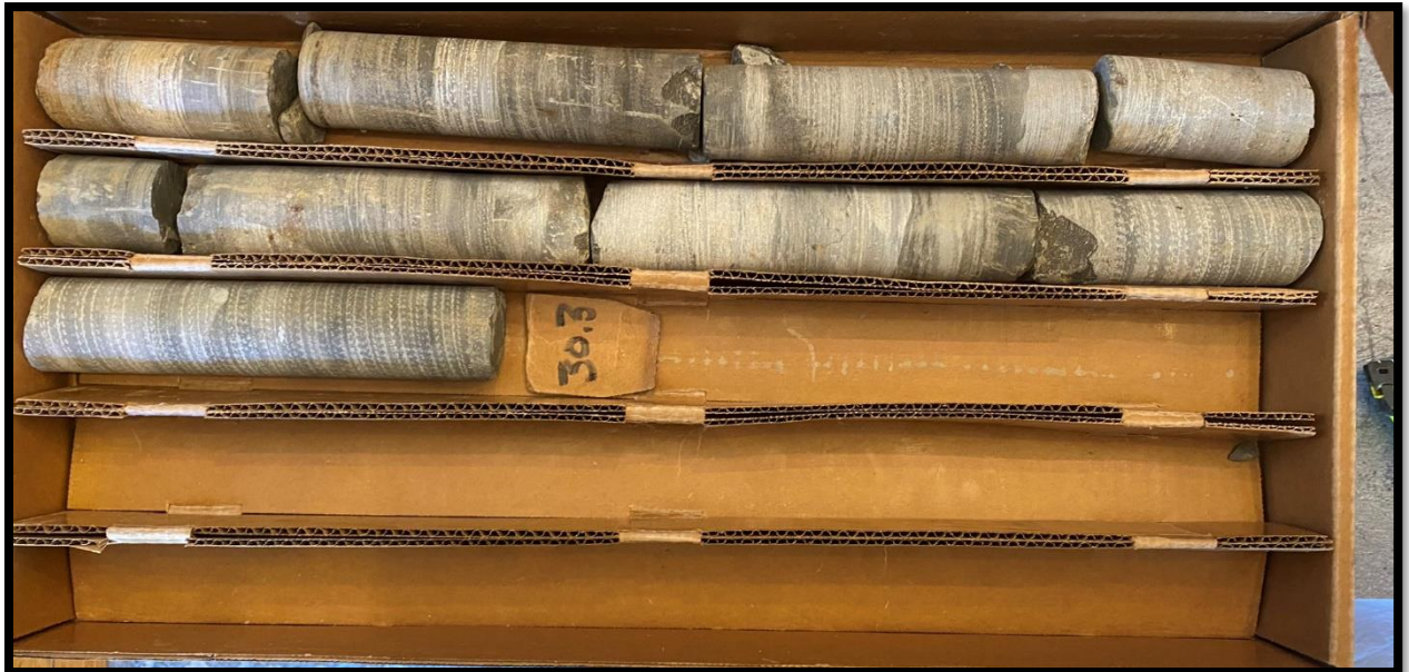
Figure 35: Boring K-16 Box 2 of 2
