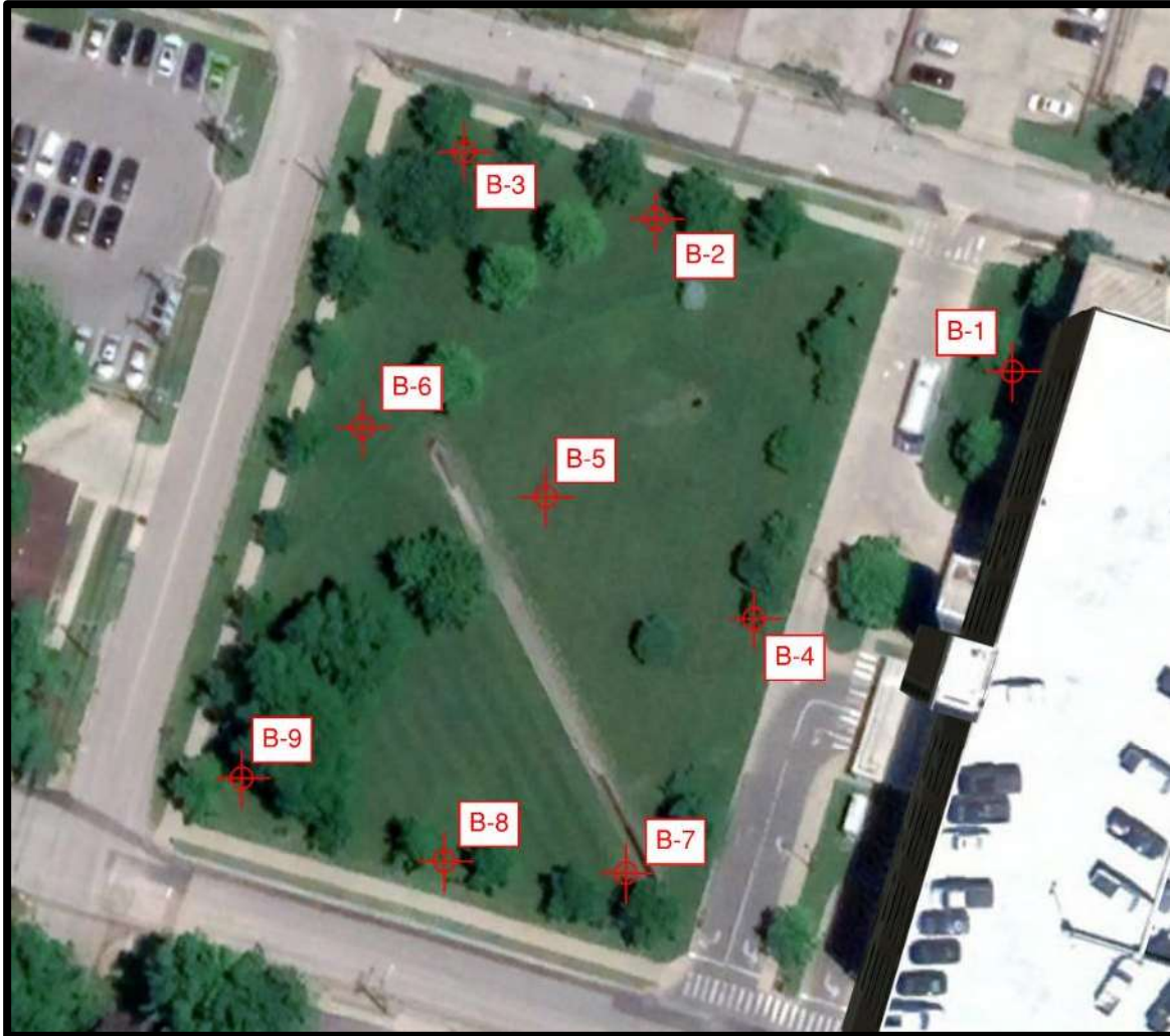
Figure 8: Approximate Boring Locations
