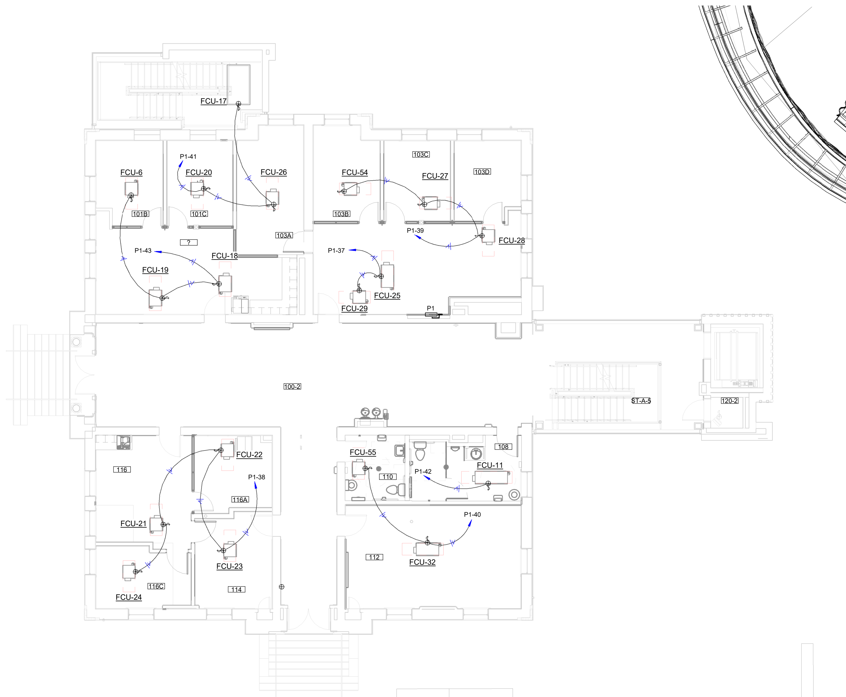
FIRST FLOOR - MECHANICAL EQUIPMENT POWER PLAN SCALE: 1/8" = 1'-0"
